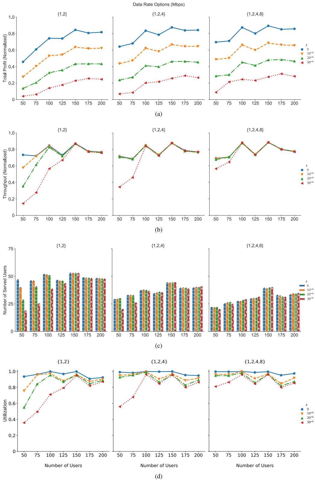
FIGURE 6. Illustration of the impact of bandwidth cost on (a) network profit, (b) throughput, (c) number of served users and (d) utilization. In the first two and last rows, the circle, downward triangle, upward triangle and leftward triangles depict 0 , 10^{-6} , 20^{-6} and 30^{-6} values of \lambda , respectively. In the third row, the same \lambda values are shown by blue, orange, green and red bars, respectively.
