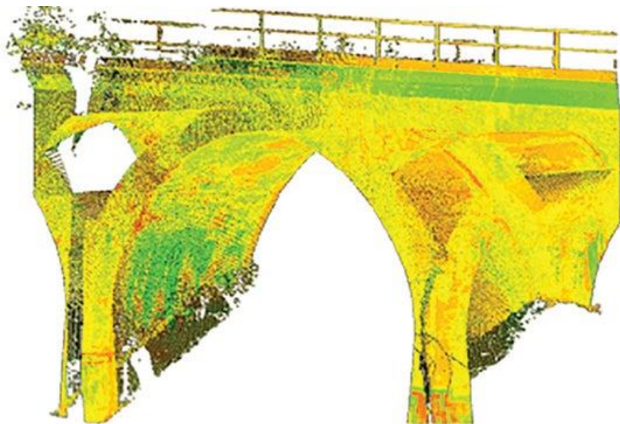
Figure 23: 3D scan of one arch. Copyright: Ingenieurbüro Dr. Sauermann – Orlicek – Rohen GmbH (Hochmuth, 2023)
