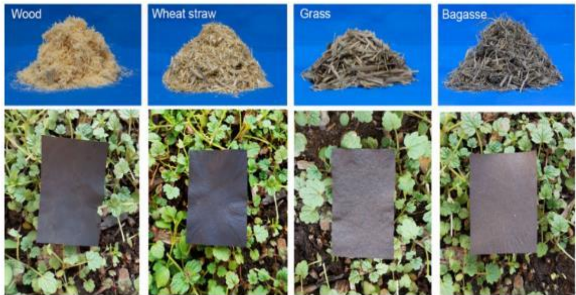
Figure 84: Lignocellulosic bioplastics' dissolving in nature changing by the derivate material (Xia et al., 2021)
